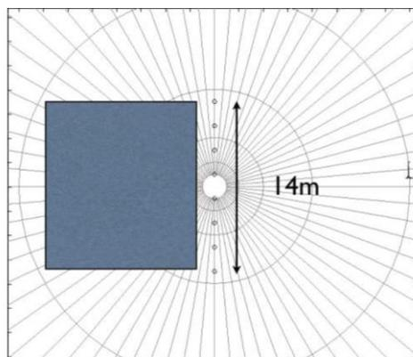
Once the subs are placed 1.70 m from each other, we will see the behavior of different frequencies to different degrees, taking the central axis as a reference. To observe the existing phase relationship in degrees we will use the formula;
