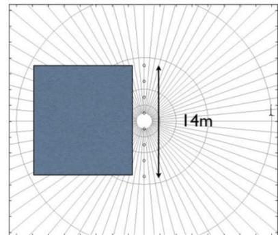
Taking the previous example as a starting point; we place the subwoofers at a distance of 1.70 m from each other and apply the following delays;
