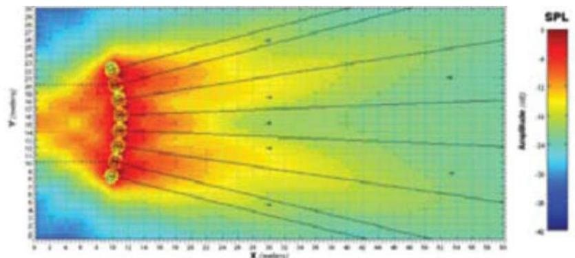
As we can see, we have gained general coverage with respect to the in-line horizontal configuration, but we have a slight reduction in level in the central area, this can be solved by placing a subwoofer above sub No. 4 and another above sub No. 5, thus recovering the level in the central zone.
